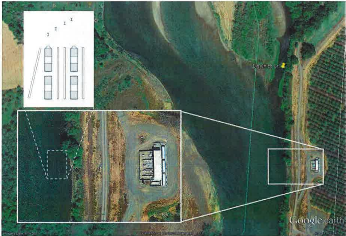
Figure 1. Location of the pumping plant and fish screen. Inset shows a plan view sketch of the screens and protective elements. The intake is on the Sacramento River immediately downstream from the confluence of Big Chico Creek. Stream flow is from top to bottom in the photos.
